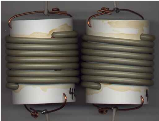
The 40 meter traps, wound on 1.5" PVC pipe couplings.
